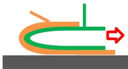
**Figure 1: 180°C Peel Test**
