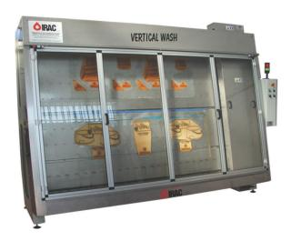
**VERTICAL WASH** Self contained washing for corrugated cliches and plates. Designed to wash all waterbased flexo inks from plates in a sealed booth so operator is never in contact with the cleaning chemical for increased OH&S.
