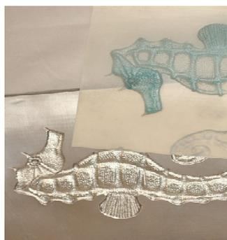
**AV 610 Epoxy Counter Die Kit** is a new and innovative way of producing professional counter dies for embossing and debossing applications.
