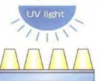
Expose the developed plate after drying again to UV light in order to get stability. Post exposure time should be the same or longer than main exposure time.
