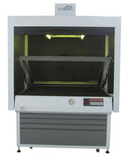
MCL ExpoMac 122E UV Exposure System is a fully self contained UV exposure and vacuum frame unit for processing photo-sensitive PE Magnesium plates. Featuring high quality, high intensity 5000w UV lamp light source, for correct exposure wavelength of 365-420NM. Includes fast vacuum integrated vacuum pumps. Complete with a strong 4 drawer base. Suitable for plates up to 850×1100mm
