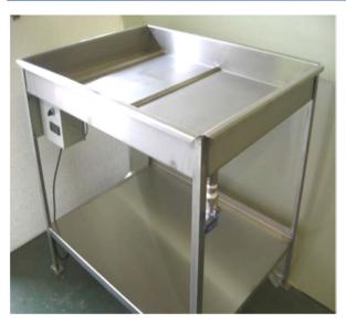
Mega Etch MA50D Developing Bath has been specially designed and built to ensure correct develop temperature when developing Luxfer PE Magnesium plates.
