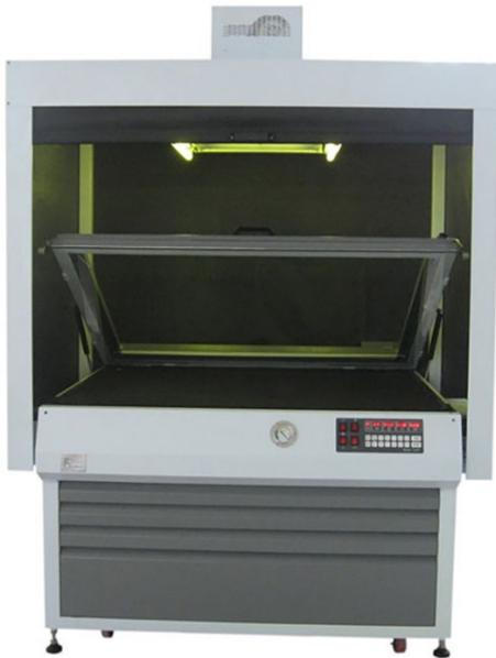
**MCL ExpoMac 122E UV Exposure System** is a fully self contained UV exposure and vacuum frame unit for processing photo-sensitive PE Magnesium plates. Featuring high quality, high intensity 5000w UV lamp light source, for correct exposure wavelength of 365-420NM. Includes fast vacuum integrated vacuum pumps. Complete with a strong 4 drawer base. Suitable for plates up to 850×1100mm
