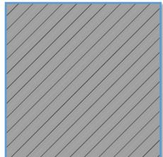
Tri-Helical Engraving. For use with tactile varnish, and glue applications or high viscosity coatings. The Tri-Helical is literally a paddlewheel for picking up and transferring high viscosity coatings. Engravings range from 40 to 250 lines per inch.
