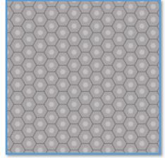
60°/30° Engraving. The six-sided cell, industry termed Hex pattern, with its ability to release more ink per square inch than its traditional mechanically engraved counterpart from years past, the 60° hexagonal shape is used for the majority of ink flexo printing applications today with engravings of 40 to 1800 LPI.
