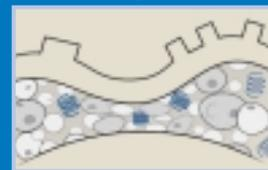
Open-cell structure "springs" recover after compression
