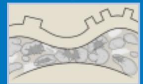
"Balloons" or closed-cell structure ruptures under over-impression
