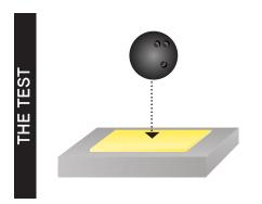
During the test, the ball is dropped on the foam and the pressure-sensing device measures the impact. It then color-codes the magnitudes of the pressures, from purple (lowest) to red (highest).
