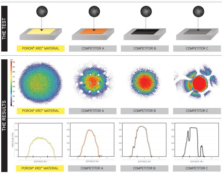
You've seen the backyard bowling experiment, now see the testing behind the demo. To measure the effectiveness of PORON® XRD™ Extreme Impact Protection Material, a bowling ball is dropped onto various pieces of foam that sit atop a pressure-sensing device. The test compared PORON XRD Materials and three other popular shock-absorbing materials used in protective equipment and apparel.
