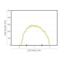
**IMPACT DISPERSION GRAPH:** The amount of pressure detected along a line through the center of the area of impact was created and mapped. The distance recorded on the x-axis is a measurement of the diameter of the impact area, and the y-axis measures the pressure detected at that distance along the line.
