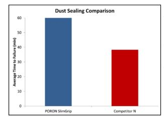
**Note:** Test materials are assembled as a 1mm wide gasket placed under 37% compression and are tumbled in a dusty environment. A material "fails" when dust penetrates the gasket.
