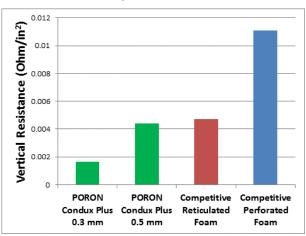
**Note:** Reticulated Foam thickness is 0.49 mm, Perforated Foam thickness is 0.42 mm. The values above represent the vertical resistance of a 1" by 1" sample under 1 KgF.
