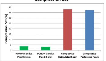
**Note:** The above graph represents typical values, tested according to ASTM D 3574-95, Test D @ 158°F (70°C)
