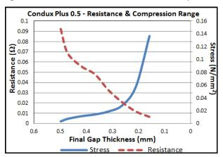
Figure 2: Condux Plus 0.5 mm Resistance & Compression
