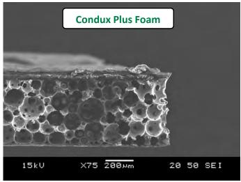
Notice the integrity of the die cut edge of Condux Plus foam above. Compare that to the collapsed, crushed edges of die cut competitive foams below.
