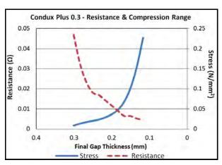
Figure 1: Condux Plus 0.3 mm Resistance & Compression
