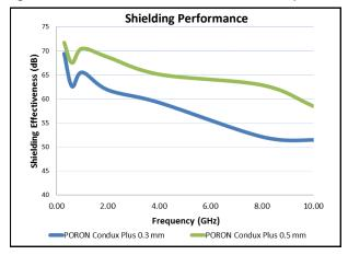
**Figure 3:** Condux Plus 0.3 mm & 0.5 mm Shielding Effectiveness Graph
