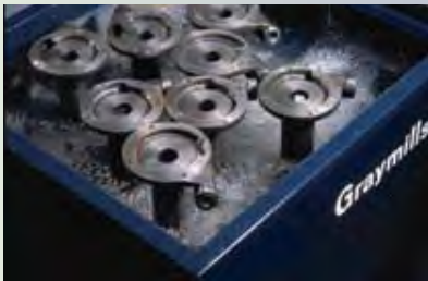
Parts are easily loaded on platform at tank top level Auto lid closes as cycle begins
