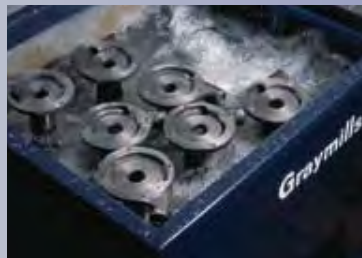
Start cycle lowers parts into solution Fully immersed parts may be soaked and/or agitated with programmable cleaning
